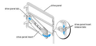
3. Ensure that the drive-panel insert is correctly seated in the drive panel.
