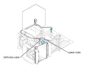
2. Press the tabs on each side of the drive towards each other and slide the drive up and out.
