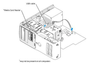
Disconnect the USB cable on the back of the Media Card Reader from the front panel USB connector on the system board (see "<u>System Board</u> <u>Components</u>") and remove the cable from the clip on the shroud. sliding plate lever
