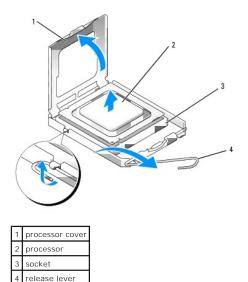
7. Release the release lever and lift the processor cover.
