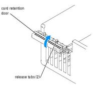
13. Close the card retention door by snapping it into place to secure the card(s).
