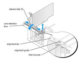
4. Push the two release tabs on the card retention door from the inside to pivot the door open. Because the door is captive, it will remain in the open position.
