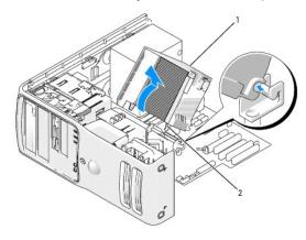
heat sink and fan shroud assembly
