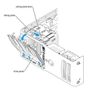
2. Grasping the lever on the sliding plate, pull the sliding plate to the right and hold in place.
