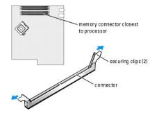
5. Align the notch on the bottom of the module with the crossbar in the connector.
